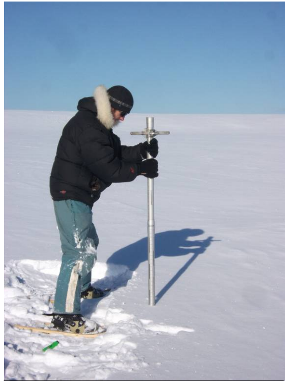
Photo 1: Staff takes a core sample to gauge moisture content and density of the snow.
